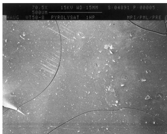
Fig. 5. SEM (70.5×) fracture surface of a PVS-derived ceramic. Prepared by densification at 200°C and 45 MPa and subsequent pyrolysis at 1050°C for 4h.
